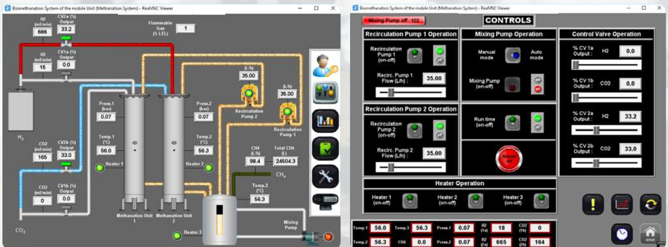
Figure 2. Programmable Logic Controller (PLC) system used to monitor and control the biological methanation reactors. The left panel shows the system's initial interface, while the right displays the configuration and control menu.
